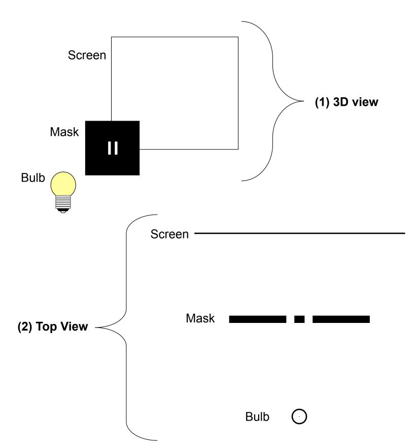
A laser is shined through two very narrow apertures (holes) in a mask onto a screen
